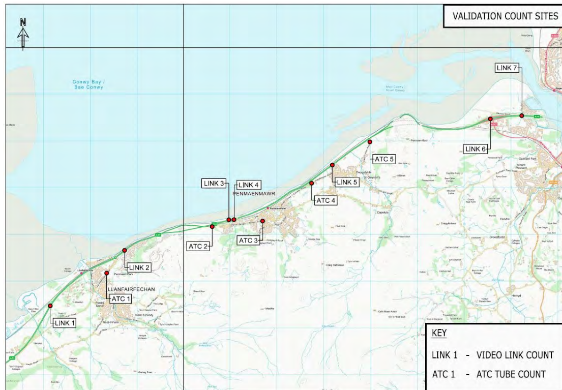
Figure 7: Traffic Counts Used in Link Flow Validation
